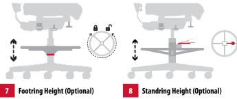
Lift the lever with one hand and raise or lower the ring with your other hand. Release the lever to lock the ring in your desired position.
